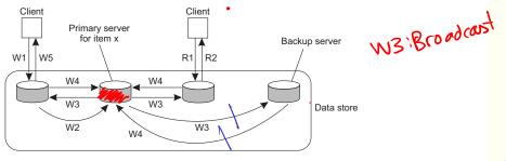
W1. Write request W2. Forward request to primary W3. Tell backups to update W4. Acknowledge update W5. Acknowledge write completed R1. Read request R2. Response to read
