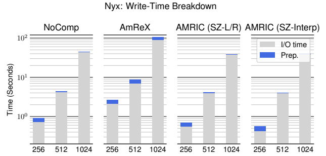
Figure 18: Writing time of Nyx runs with different scales. Log scale is used for better comparison.
